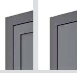
Strong profile: Everything Frame and sash in line: Frame arranged offset and sash are flush with one another
